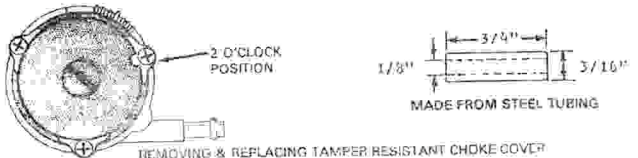
REMOVING & REPLACING TAMPER RESISTANT CHOKE COVER FIG. 1
